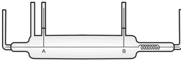
Fig. 3 Schleiermacher's hot wire instrument [20]
